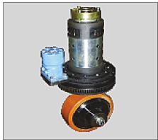
Integrated structure of drive system and steering system.
