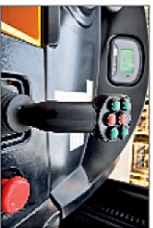
Control handle with integrated thumb stick, allows smooth operation of (1) Travel, (2) Lift/low, (3) controls Tilt and Fork Reach.
