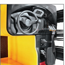
Large cab with dead man power off switch, Multi-function display, battery state, hour meter, fault indicator etc.
