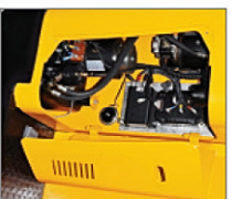
Vertically mounted drive motor with CANbus technology reduces wiring complexity and increase reliability.
